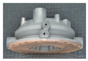
manifold made of oxidation-resistant nickel-based superalloy Monel K500. GRCop-42 allows propellants to effectively cool the injector face while the oxidation resistance and strength of Monel K500 allows thinner walls in the manifold, resulting in a lighter design solution tailored to the demands of RDRE applications.
